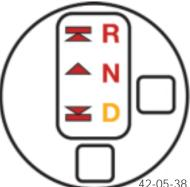
**Position P** is separate from the actual shift pattern. P is indicated in the instrument cluster only when the park position is engaged and the ignition is "ON".
